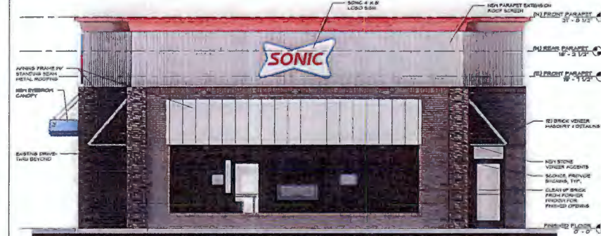
2 RENOVATED FRONT ELEVATION 1/4" = 1'-0"
